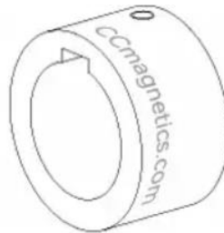
Type B with feather keyway and setscrew
